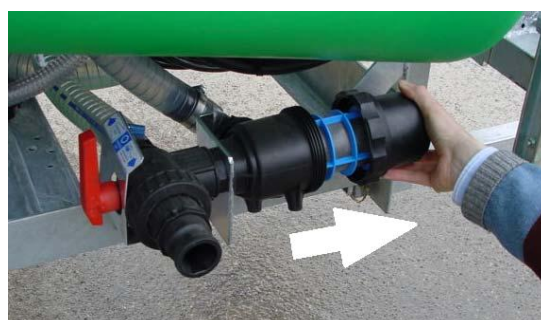
Dismantling the Suction Filter
